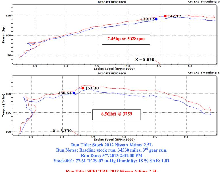
Run Title: SPECTRE 2012 Nissan Altima 2.5L Run Notes: SPECTRE intake kit #10233 installed. 34530 miles. 3<sup>rd</sup> gear run. Run Date: 5/7/2013 3:14:20 PM SPECTRE.002: 79.78 °F 29.03 in-Hg Humidity: 15 % SAE: 1.02
